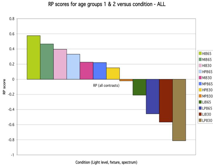
**Figure 7:** The Reading performance is affected by three factors – light level, spectrum and light distribution. The best reading performance is at the high and medium light levels with the 865 lamp/indirect luminaire combination while the worst reading performance is under the 830 lamp in the indirect and parabolic luminaire.
